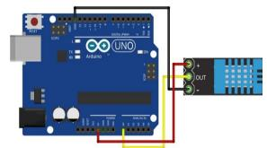
Fig. 10. Connection Circuit of Temperature and Humidity Sensor
