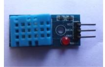
Fig. 9. Temperature and Humidity Sensor
