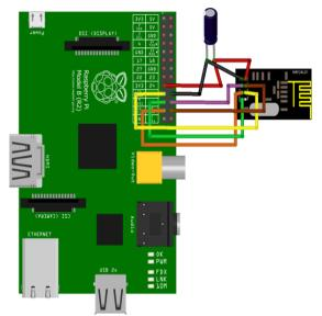
Fig. 3. nRF24L0+1 Wireless Transceiver connects to Raspberry Pi 2
