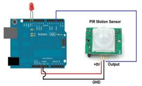
Fig. 7. Connection Circuit of PIR Motion Sensor
