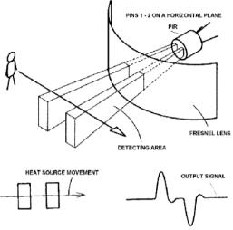
Fig. 8. The Motion Detection by PIR Sensor within the system.
