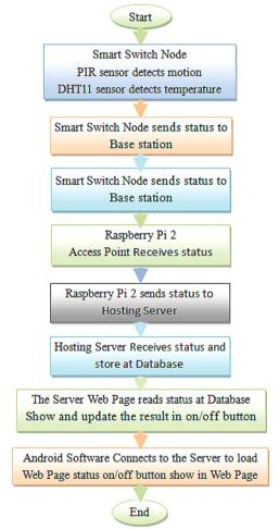
Fig. 12. Flow chart for smart switch node sends status to Android app.
