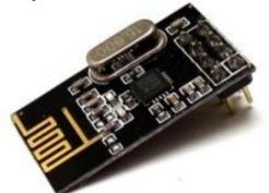
Fig. 4. The nRF24L0+1 Wireless Transceiver
